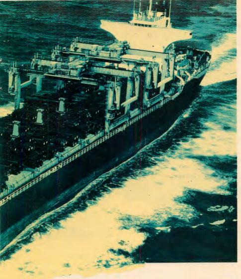
Saving space by separate shipment, SS Pittsburgh carries wheeled chassis for hauling containers by tractor/trailer. Photo: Skyfotos
